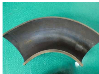
Figure 6 Longitudinal section of the existing elbow
