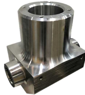
Figure 13 Finished valve body
