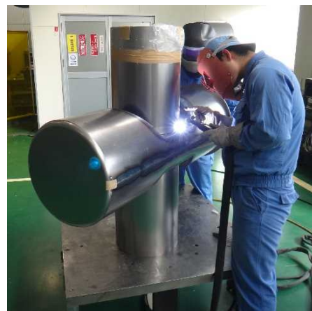
Figure 5 Assembling of the capsule
